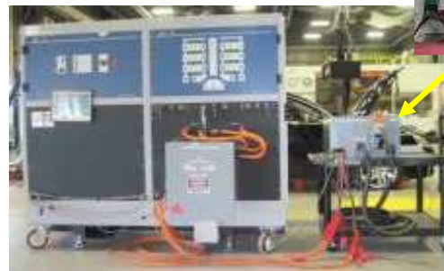
AC/DC Charging Comm. Controllers: SAE J2931/4 (HGP) with CAN/Ethernet Ports
