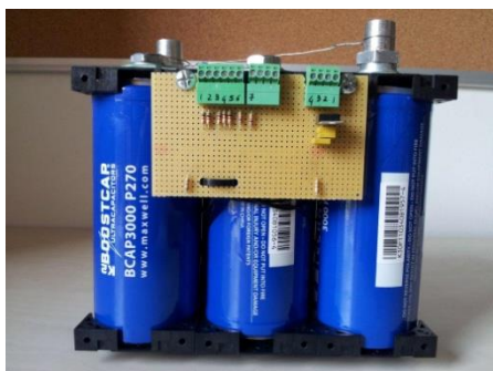
Figure 4: SC module (16.2V, 500F, 5.9 kW/kg) supplied by DimacRed
