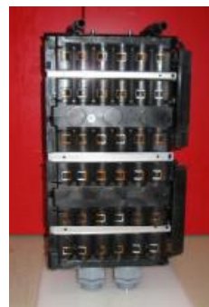
Figure 5: Li-ion module (8,5 Ah, 59,4 V, 505 Wh, 11,25 kW, about 10 kg) with cover prepared by Magna e-car
