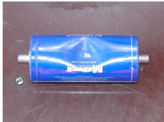
Figure 10: SC cell deformation after crush test
