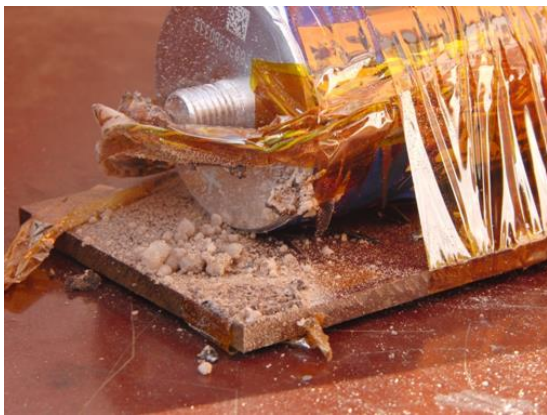
Figure 12: Cell after thermal stability test. Release of electrolyte through hole in casing
