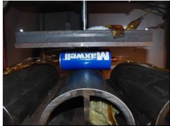
Figure 9: Maxwell SC in hydraulic press for Controlled Crush Test
