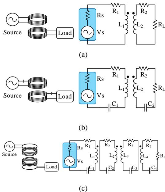
Figure 1: Topologies and equivalent circuit models of near-field wireless power transfer technologies: (a) traditional IPT; (b) coupled magnetic resonance; and (c) strongly coupled magnetic resonance.
