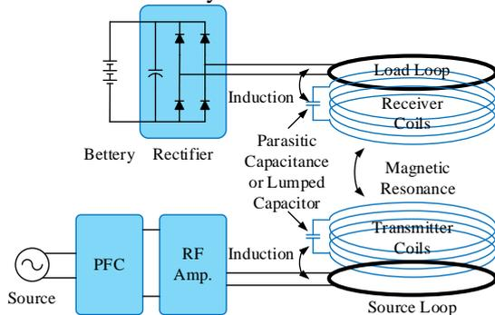
Figure 2: Schematics of strongly coupled magnetic resonance wireless EV charging system.
