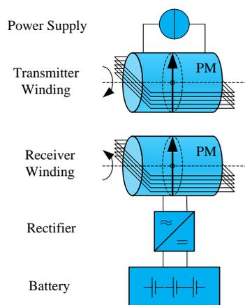
Figure 3: Schematics of magnetic wireless EV charging system.
