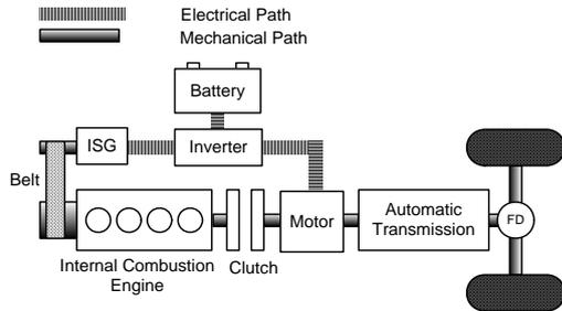
Figure1: Parallel HEV configuration
