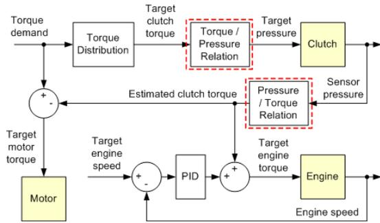
Figure5: Control scheme of the launch slip engagement
