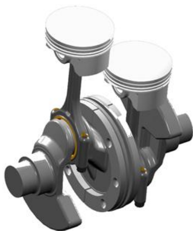
Figure 2: Two bearing crankshaft arrangement with a central flywheel
