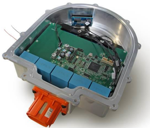
Figure 3: complete 3-phase inverter system used for comparison of 650V and 400V IGBTs technologies
