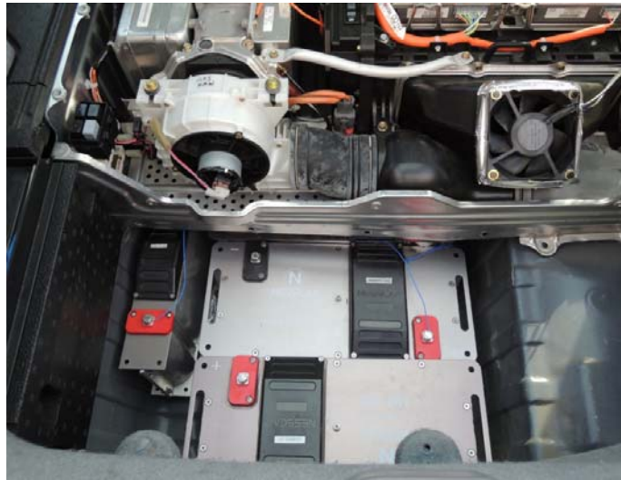
Figure 3: Rear section of the Insight showing the electronics and ultracapacitors in the storage compartment
