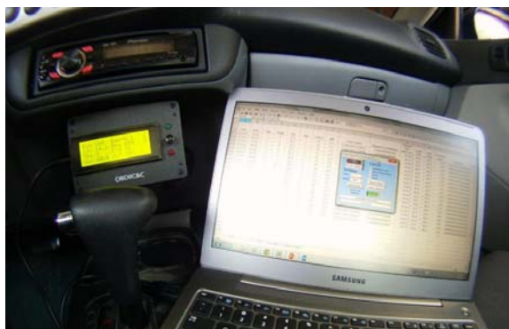
Figure 5: OBD readout (left) and laptop running PLX-DAQ Data Acquisition Software (right) logging data during a vehicle drive.
