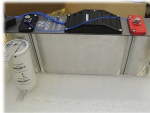
16V module (6 x 3000F cells)
