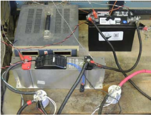
Figure 7: Laboratory test set-up for the micro-hybrid arrangement
