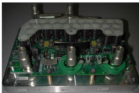
Figure 1. The pictures on the left and in the center show a motor control unit with E-Cap-Bank, courtesy of Curtis Instruments Inc. The diagram on the right shows the dimensions of the model LXZ 63V 820 capacitor used in the unit.
