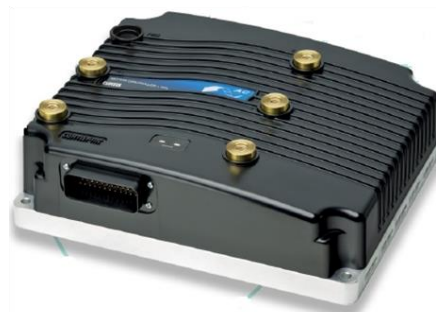
Figure 1. The pictures on the left and in the center show a motor control unit with E-Cap-Bank, courtesy of Curtis Instruments Inc. The diagram on the right shows the dimensions of the model LXZ 63V 820 capacitor used in the unit.
