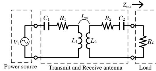
Figure 2: Equivalent circuit of magnetic resonant coupling with power source and load
