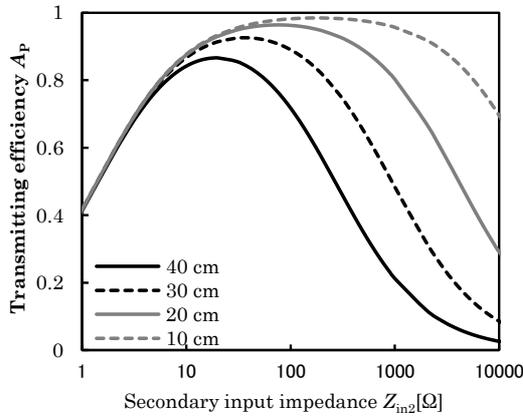
Figure 4: Relation efficiency and load resistance
