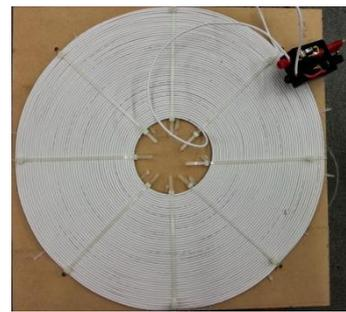
Figure 3: An antenna for Wireless power transfer
