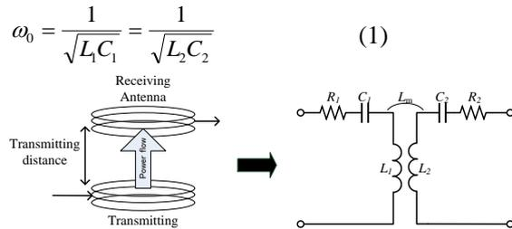
Figure 1: Equivalent circuit of magnetic resonant coupling
