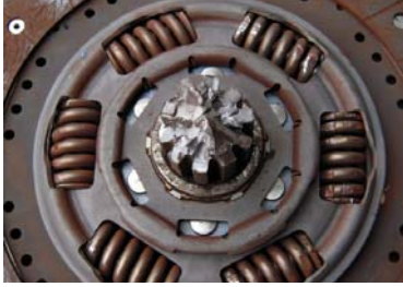
Figure 1: A broken shaft in the clutch
