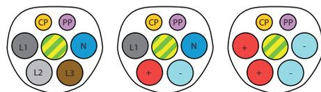
Figure 8: Combined use of Type 2 connector: three phase a.c., single phase a.c. with d.c., d.c.
