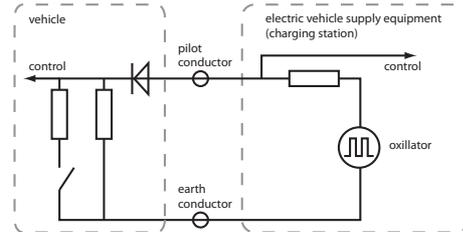
Figure 1: Control pilot conductor
