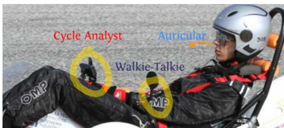
Figure 1: Electric vehicles of the University of Malaga with the previous speech system for data and advice feedback.
