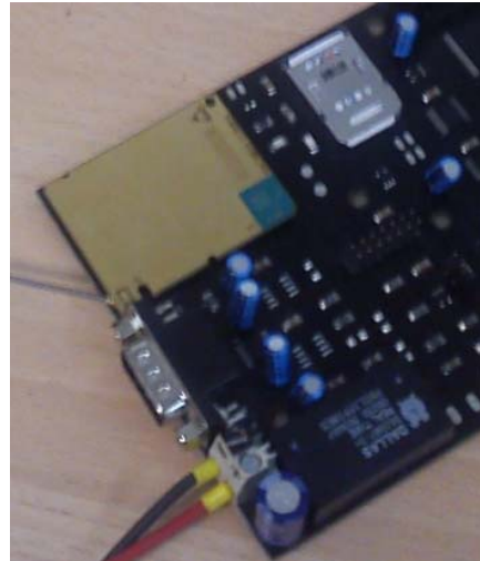
Figure 4: Telemetry electronic system: Electronic controller.
