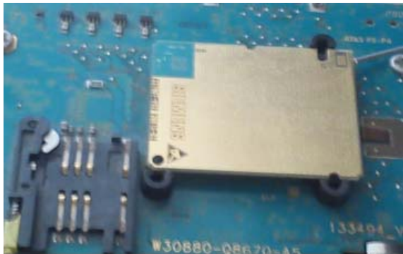
Figure 5: Telemetry electronic system: TC-65i.
