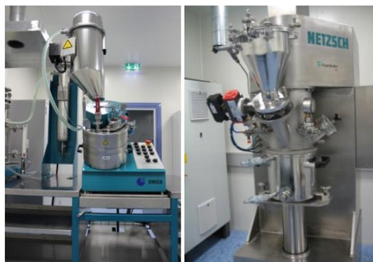
Figure 2: Intensive mixer and planetary mixer used for mixing investigation.
