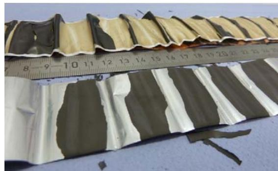
Figure 1: Post mortem analysis of a commercial consumer battery.
