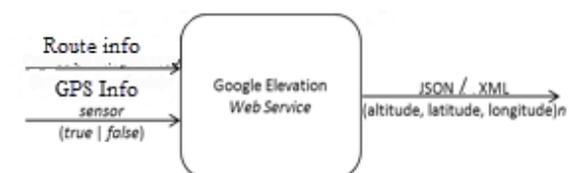
Figure 5: Determination of the path altimetry.
