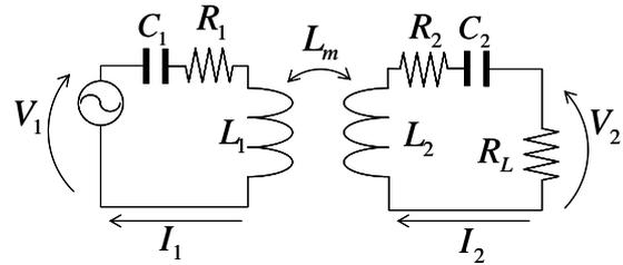
Figure 10: Equivalent circuit of single phase system
