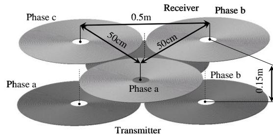
Figure 1: Setting of resonators
