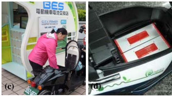
Figure 4. The procedure of swapping lithium ion battery [5]
