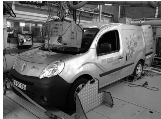
Figure 6: FlexHybrid prototype on a vehicle test bench
