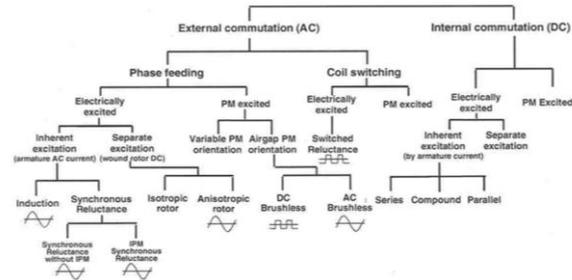
Fig. 1 Electrical machines and wave forms of the related electric drives
