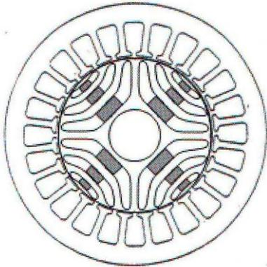
Fig. 2 Synchronous reluctance machine with permanent magnet compensation.
