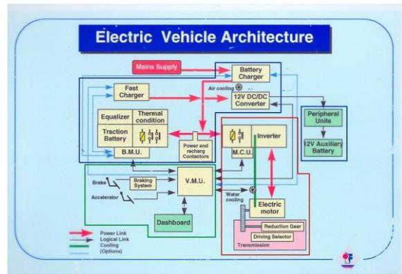
In the schematic the areas are identified related to Energy Storage and charge, Power train, Energy Storage and Communication and Peripheral Units.
