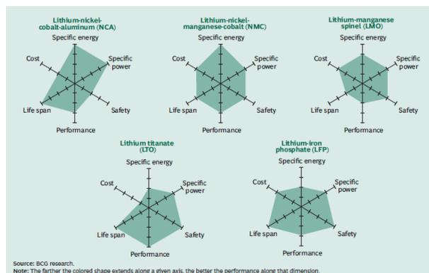
Fig. 5 Parameters tradeoff for the different types of lithium-ion batteries
